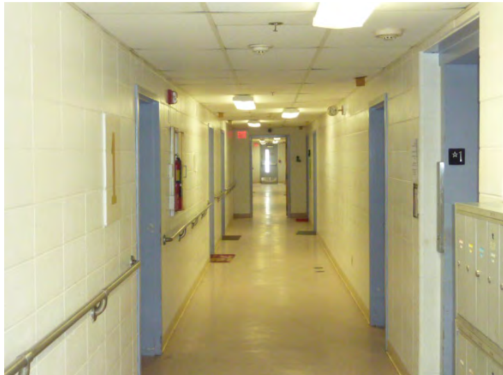
Typical corridor with ceiling and wall mounted call for aid lights, sprinkler heads, emergency lights, fire extinguishers, smoke detectors, fire alarms and exit signage.
